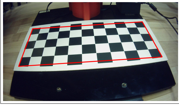
Fig. 4: Distorted image taken by a fisheye lens camera
